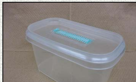
Figure 2. Microbox vessel with microporous filter.
