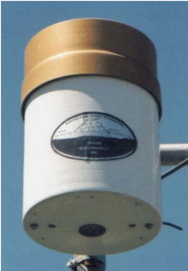
Figure 5. A tipping bucket rain gauge used to measure precipitation.
