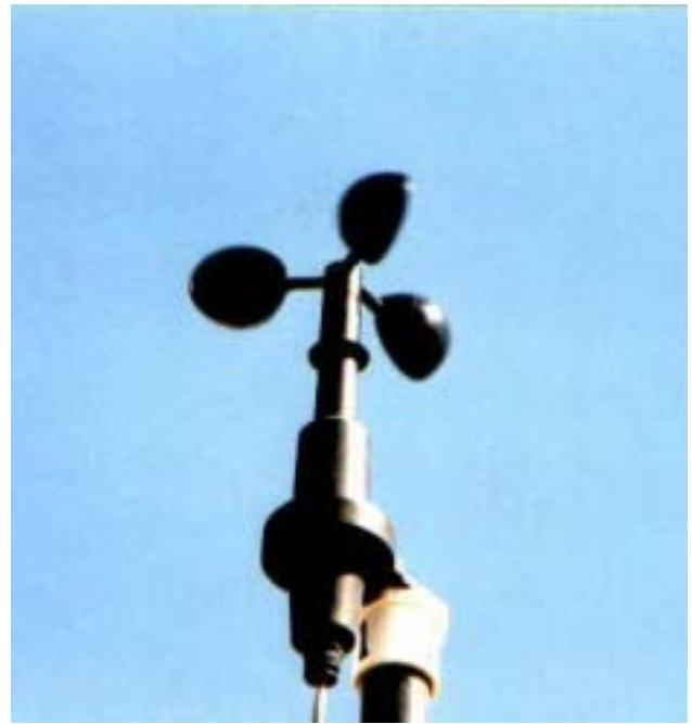
Figure 4. Anemometer (above) and wind vane (below) commonly used on automated weather stations.
