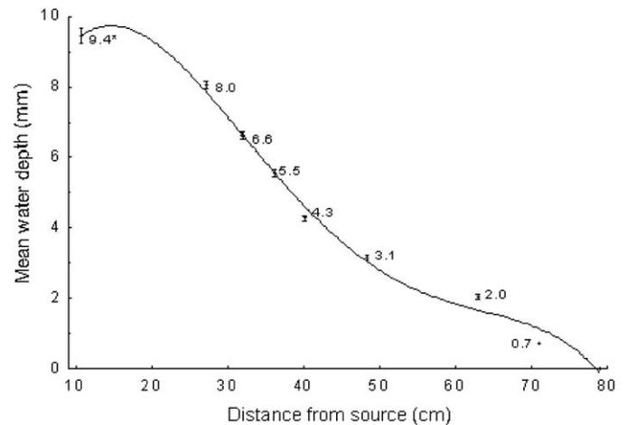
FIGURE 1. Mean depth of water (mm) per day ( $\pm$  SE) applied across a range of distances (cm) from the line-source irrigation system (LSIS). Positions used in experiments are labeled with mean depth of water (mm). Observations fitted with a fourth-order polynomial;  $y = 4.6323 + 0.8094x - 0.0399x^2 + 0.0006x^3 - 3E-06x^4$ ;  $r^2 = 0.9942$ .
