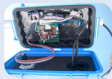
Figure 1: The "brain box" of a Snowcloud node. The brain box includes a sonar emitter/receiver, sensor control board and a connection to an external antenna for data transmission.
