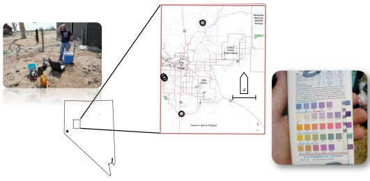
Figure 1: Left: shock chlorination experiments being conducted in the field. Center: Location of study area, with locations of test wells indicated in circles; Right: simple chlorine test strips used as an indicator of adequate purging
