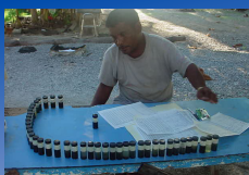
A worker logs results from H 2 S tests on water from local rainwater catchments.
