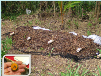
Figure 1. A passive composting pile in Tinian, equipped with an aeration system. Hobo® Tidbit temperature dataloggers (inset) were installed in the piles in three horizontal transects (which formed two full vertical transects) which provided information about temperature distributions in the bottom, mid and top fractions of the pile.
