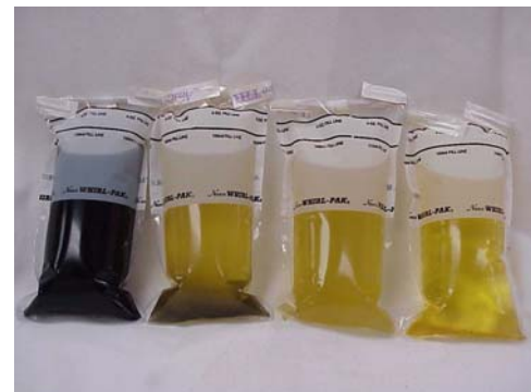
The two kits on the left (black and brownish) are positive. The two kits on the right (turbid and clear with light precipitate) are negative.
