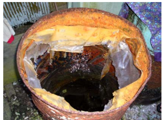
Metal drums, even when lined with thin plastic, do not make good catchments because bits of plastic, metal, and paint leach into the water.
