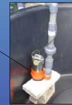
1/2 hp submersible water pump (25psi)
