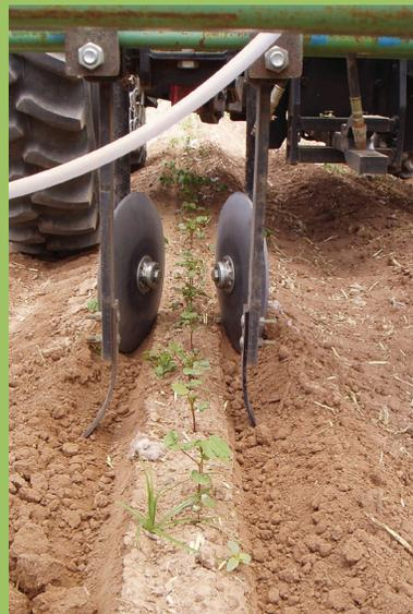
Closer mechanical cultivation to the cotton seed line reduces herbicide requirements with real time kinematic global positioning system (RTK-GPS) technology. Related research is underway at the University of Arizona's Maricopa Agricultural Center.
