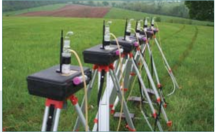
Air samplers at work in a field near Leesburg, Virginia.
