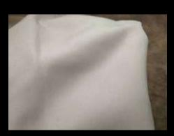
Hardline® - Hardline® is a fabric made of AlliedSignal's Spectra® fiber. It is a distinctive looking, high-tenacity nylon fabric with a super strong white Spectra fiber grid interwoven as a ripstop. Hardline fabric is used for rugged footwear, ski gaiters and other technical outerwear.
