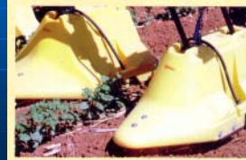
Streamlined design of the Spray-Hoods allow them to glide gently between crop rows. This limits contact with crop and provides for faster travel speeds.
