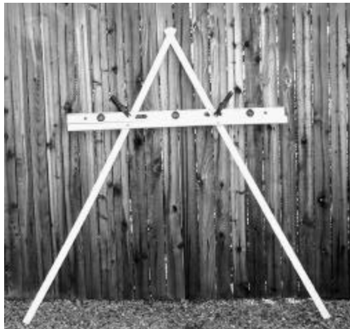
Fig.1 Completed A-frame Contour Finder
