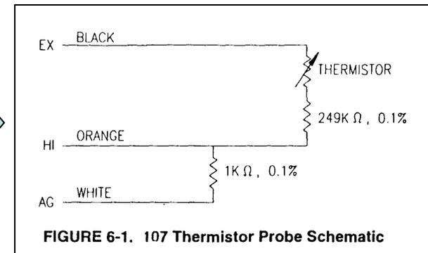
Thermistors are temperature sensitive electrical resistors. They are typically placed in a simple half bridge electrical circuit. As the temperature changes, the voltage drop across the thermistor changes and is measured by a data logger or voltmeter.
