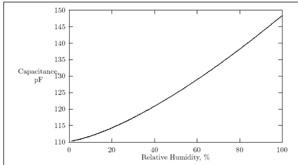
**Electrical Capacitance of Sensor Changes With Humidity. When Sensor Is Installed In Proper Electrical Circuit, Voltage Output of Sensor Changes Linearly With Humidity. The Voltage Is Measured With The Data Logger**
