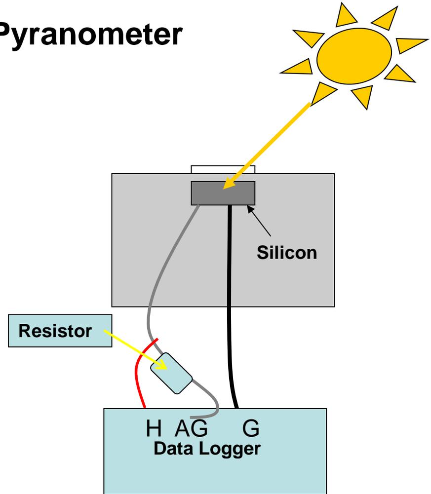
Silicon cell converts solar energy into an electrical current. The current is forced across a resistor to generate a voltage drop which is measured by the data logger.
