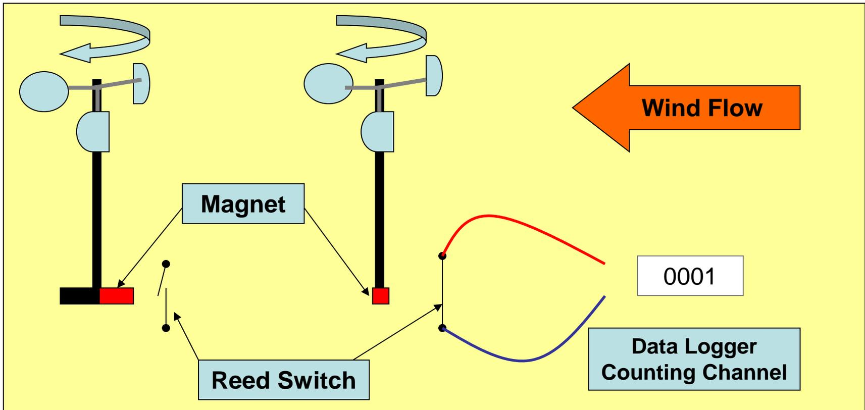
Wind rotates cups and attached magnet which is located adjacent to a reed switch. The rotating magnet opens and closes the switch. The data logger counts the number of switch closures over a defined period of time.
