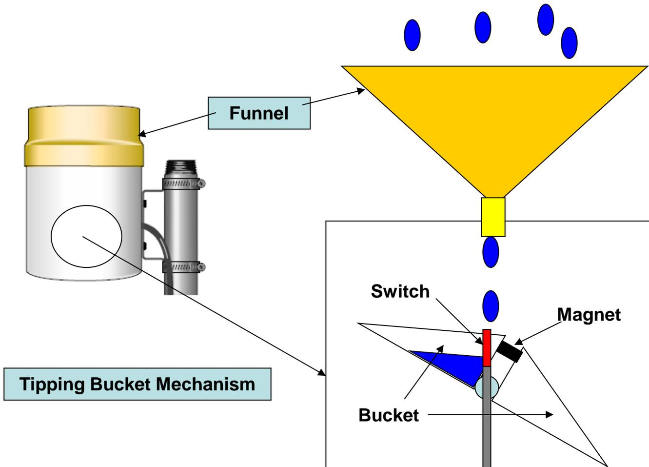
Funnel directs rainfall into tipping bucket mechanism. When one bucket accumulates 0.01" of water, the mechanism tips which causes the magnet to trip a small switch. This switch closure is counted by the data logger as 0.01" of precipitation.
