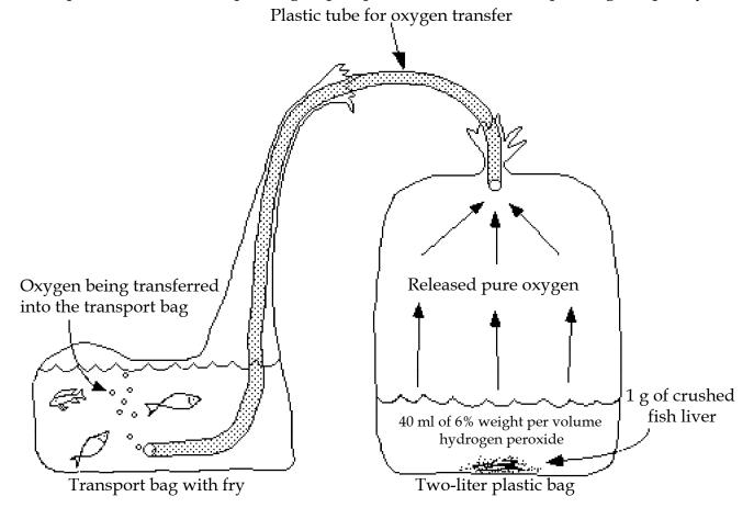
Figure 19: Producing pure oxygen from hydrogen peroxide for fish transport.
