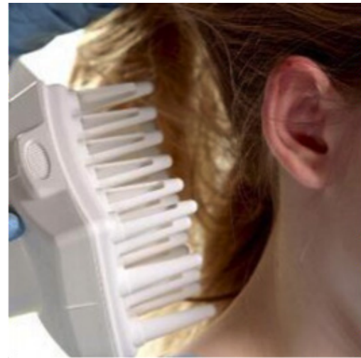
Figure 9. The machine uses hot air to desiccate lice and eggs. Image: AirAllé™
