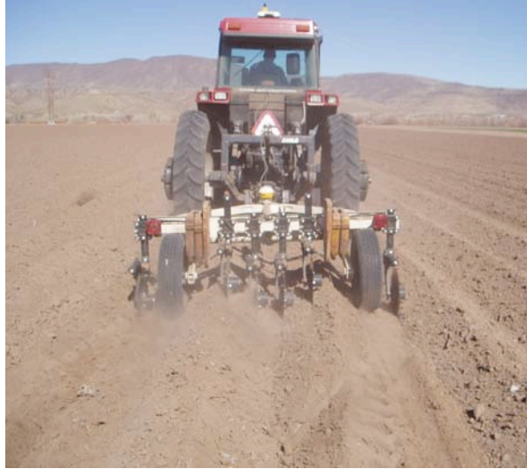
Veris sensor. Apparent Electrical Conductivity (EC a )
