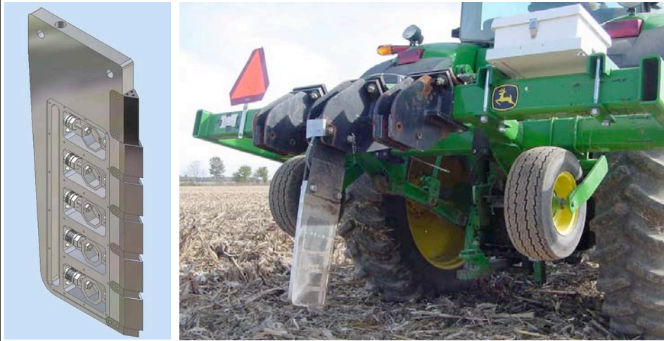
UCDavis soil compaction profile sensor
