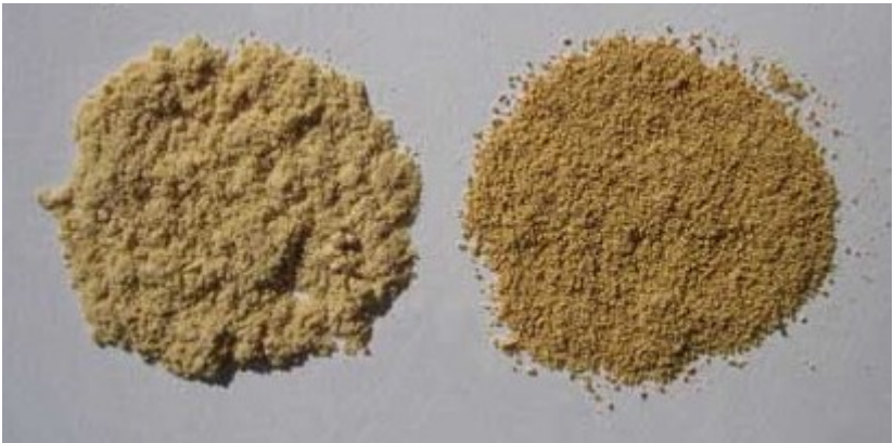
True powderpost beetle frass (left); deathwatch beetle frass (right) Photo: Robin L. Tabuchi, University of California, Berkeley
