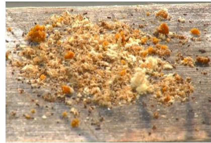
Carpenter bee damage-note the neat circular hole with fecal stains outside (left)-Photo: Tony Alter; Wood shavings mixed with pollen and other debris, seen below the hole (right)- Photo: PixOnTrax
