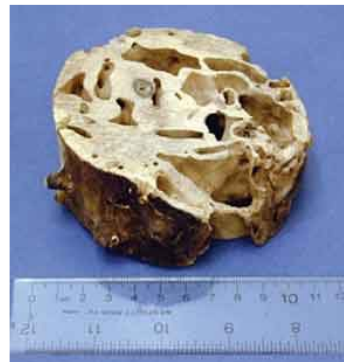
Western drywood termite damage
