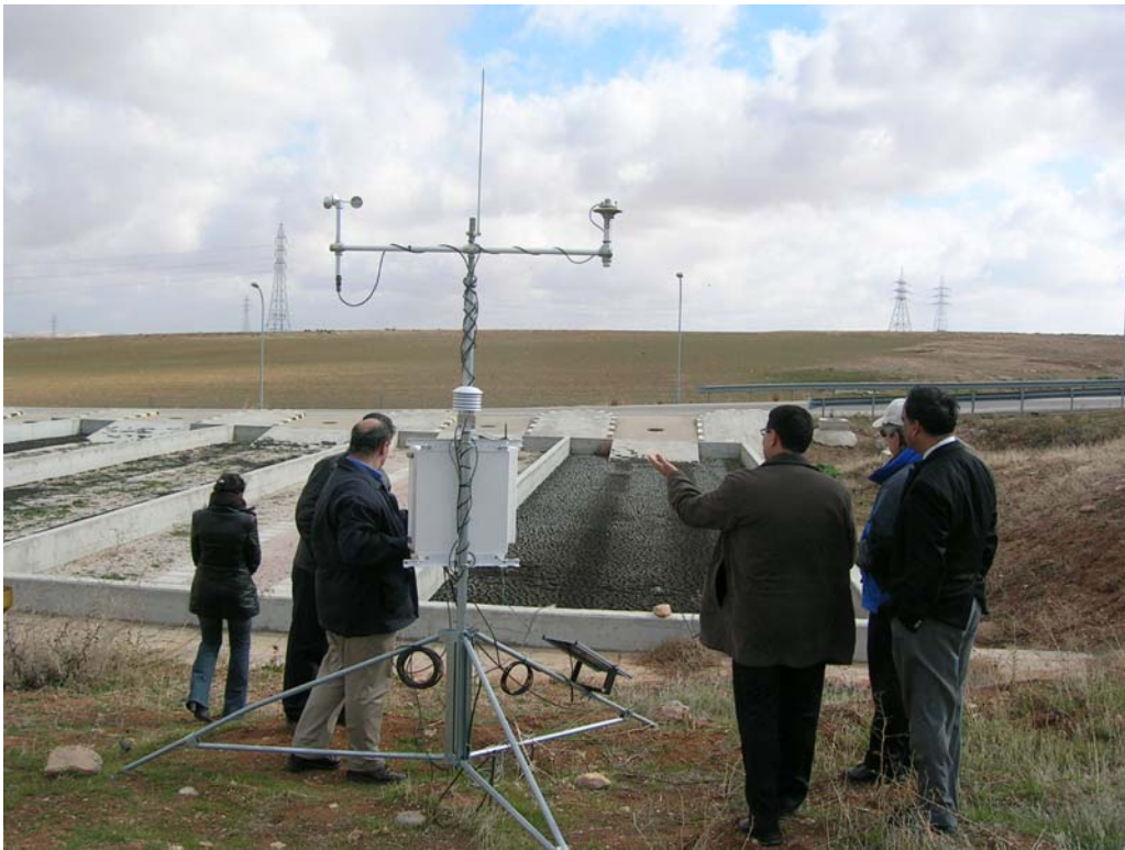
Photo 4: Biosolids drying beds with meteorological sensors to measure factors affecting the quality of treated Biosolids.
