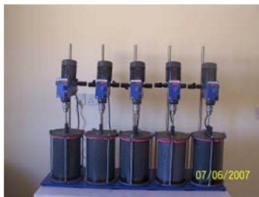
Figure 1. first set of reactors operated at five Different mixing velocities and at 60d of SRT
