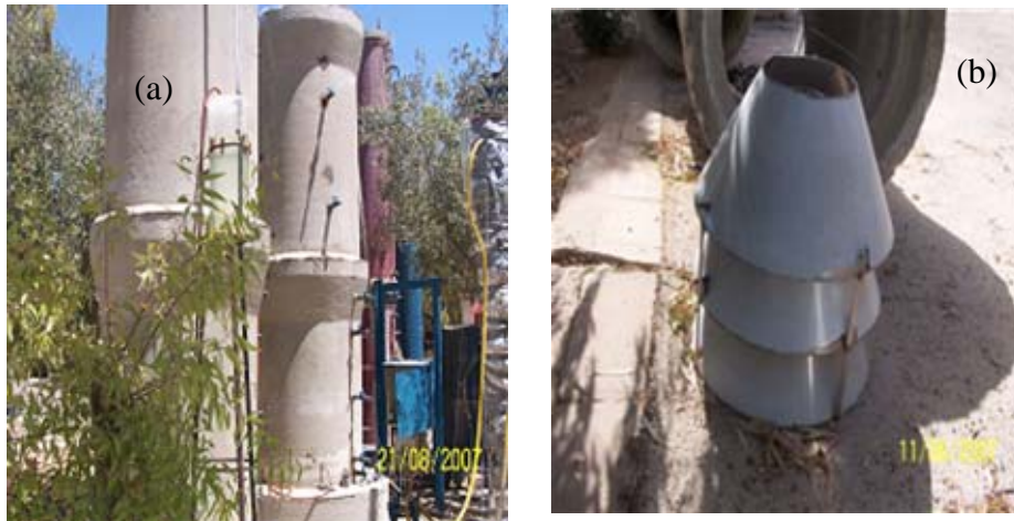
Figure 3. Two UASB reactors (a) with GLS layers (b) installed at the location of Abu-Busier wastewater treatment plant.
