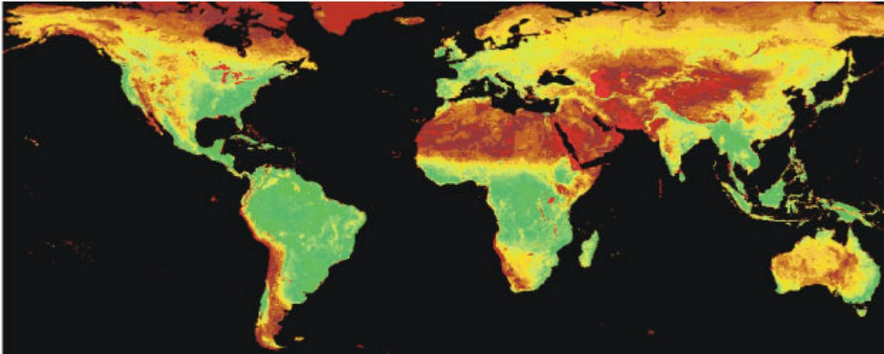
Figure 1 : A Global NDVI Image. This image was produced by taking the first principal component from a series of 36 monthly images from 1986 through 1988. As such, it represents the characteristic NDVI over the entire period for each region.
